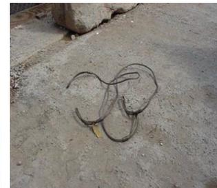
Defective wire rope sling in Yard
