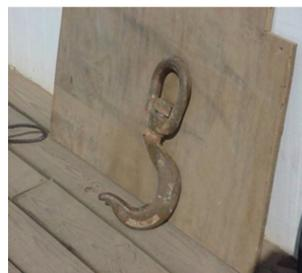
Defective lifting hook
