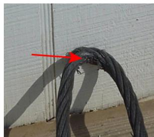
Damaged wire rope sling in shipping area
