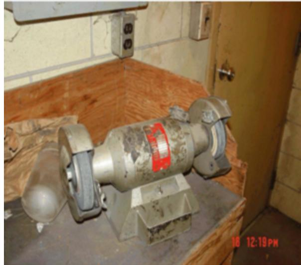
Grinder should be mounted to work bench and guards installed
