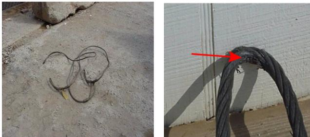
Defective wire rope sling in Yard    Damaged wire rope sling in shipping area
