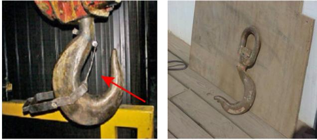
Safety latch is broken - East bay    Defective lifting hook
