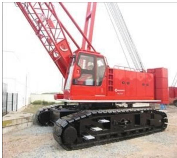
Radius guard is missing on this crane
